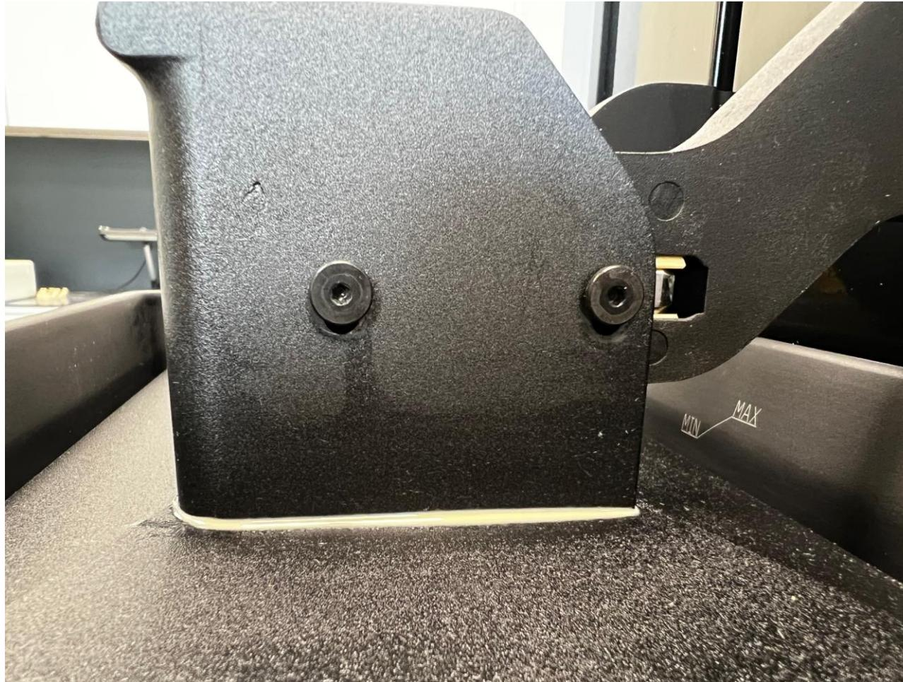
Use arrow (1x = 0.1mm \ 2x =1mm) to move build platform down until screws in slotted hole move to center (see following 2 pages!!!)
